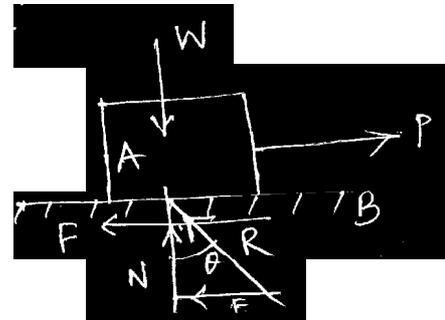
Let R be the resultant reaction between normal reaction and force of friction acts at angle  $\theta$  to the normal Reaction.  $\theta \rightarrow$  Angle of friction.
