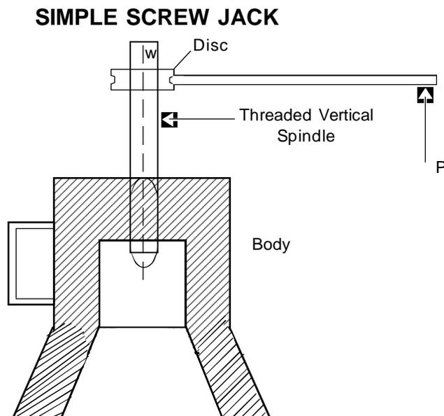
A Simple Screw Jack consists a vertical threaded spindle. The threaded portion of the spindle passes through a nut cut in the body of the Screw Jack.
