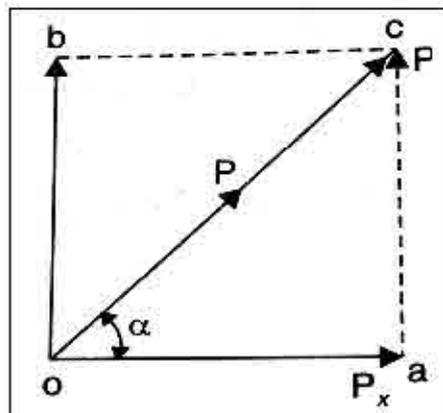
Let  $P_x$  is the component of force P in the direction oa making an angle ' $\alpha$ ' with the direction oc.
