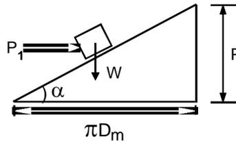
Let  $P_1$  = horizontal force required to move a body of weight  $W$  up the inclined plane.
