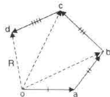
If the forces  $P_1, P_2, P_3$  and  $P_4$  acting simultaneously on a particle be represented in magnitude and direction by the sides  $oa, ab, bc$  and  $cd$  of a polygon respectively, their resultant is represented by the closing side ' $do$ ' in the opposite direction as shown in the figure.
