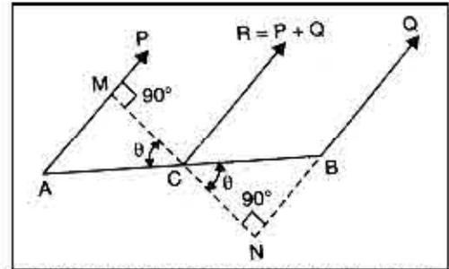
The moment of R about C is zero, so that the algebraic sum of moments of P and Q about C, must also be zero.
