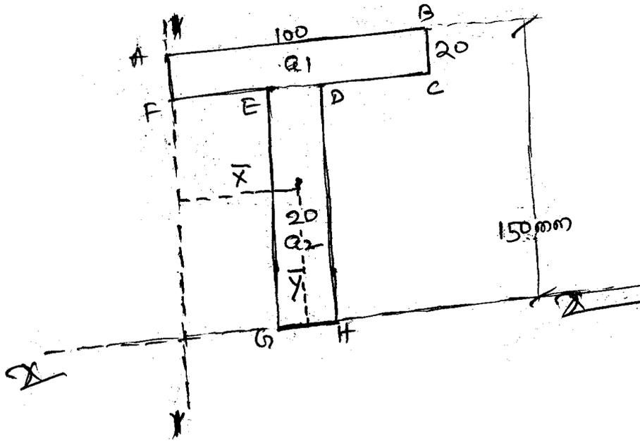
Two reference axes are selected i.e. y-y and x-x at the extreme left and bottom of the given section.
