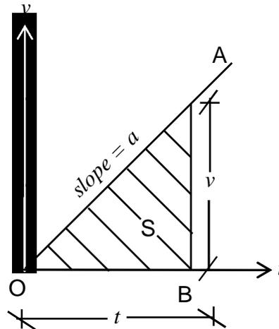
From geometry of the figure we may write  $v = at$  ----- (1),  $s = 1/2 vt$  ----- (2)
