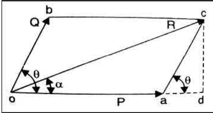
From the geometry of the figure  $\angle cad = \theta$ ,  $ac = Q$ .
