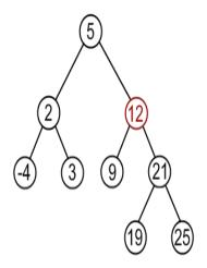
2. Find minimum element in the right subtree of the node to be removed. In current example it is 19.
