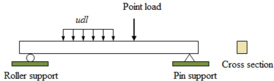
Fig.6 Loaded beam
