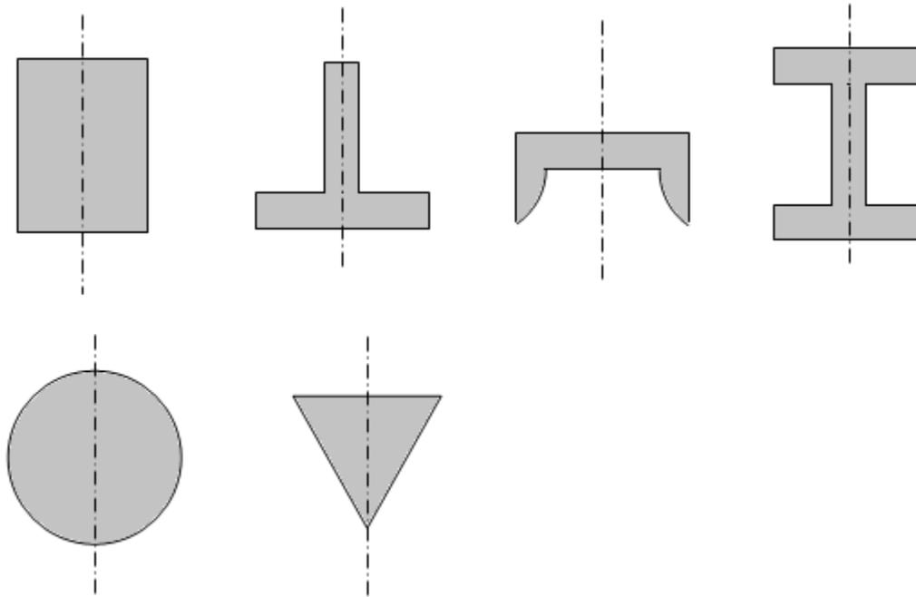
Fig.5 Beam cross-sections with vertical axis of symmetry
